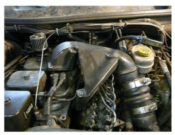
1. Remove air-intake horn by removing (5) 10mm bolts, (1) 10mm dipstick bolt, and loosening (1) 7/16" t-bolt clamp on the air-take hose. Take care when removing the intake horn to not damage the gasket at the mating surface, normally this gasket can be reused, but if it is damaged a replacement is available from Cummins, part number 3913352.
