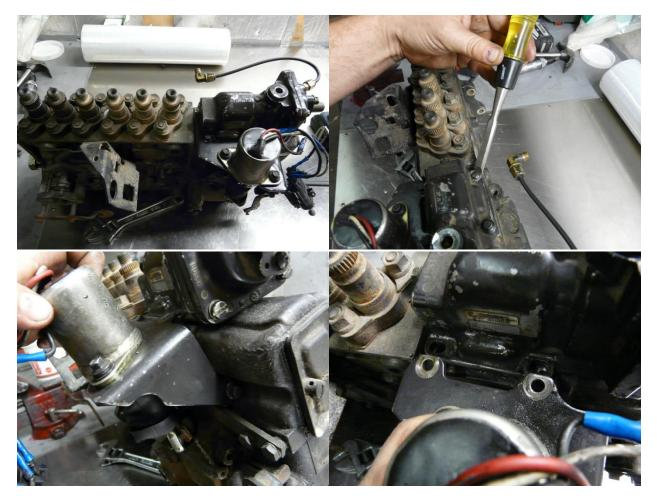
11. Remove the fuel plate being careful to not drop screws or washers into the open governor housing. If the fuel plate is left installed, it will limit injection pump fueling long before the AFC reaches full travel. This AFC Max Travel Kit is designed to provide full AFC foot travel, therefore fuel plate removal is recommended. **It's advisable to use a magnet when removing the screws.**
