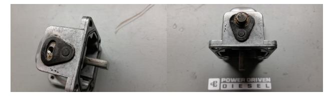
17. Remove the 5/16" or 8mm allen socket plug on the top of the AFC to gain access to the star wheel. If this plug has never been removed, it will be pretty tight and may require a vise to hold the AFC when breaking it loose. (It's regular standard thread: righty-tighty, lefty-loosey)
