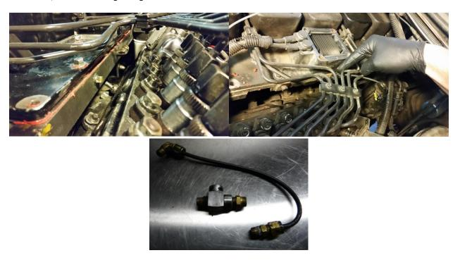
3. Install the two new 90° composite fittings (provided in the kit), one in the cylinder head and one in the AFC threaded hole where the stock fittings were removed in step 2 above.
