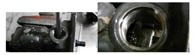
19. Discard the cupped washer and stock AFC spring. Install the new Power Driven AFC spring, then the smaller washer followed by the larger washer provided in the kit.
