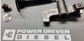
15. Using a grinder or cut-off wheel, remove 1/8" (0.125") from the guide barrel of the AFC foot, for maximum AFC foot travel a minimum 0.100" must be removed. Optional: lightly grind the face of the AFC foot to remove the reverse/negative rake on the upper portion of the foot. The dark portion of the foot face in the picture is left stock, only the upper half is lightly ground flat to remove the upper reverse rake.
