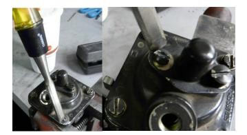
13. Under the AFC back cover is a red rubber-like diaphragm. Remove the 10mm nut, small washer, large washer, diaphragm, inner cupped washer, and stock AFC spring.
