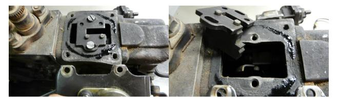
12. Take the AFC to a suitable working location (work bench). Remove AFC cover by removing (3) flat-standard screws and grinding a slot in (1) tamper-proof screw and then removing screw. Also grind a slot in the tamper-proof screw on the small pre-boost fuel cover and remove the cover. A sharp chisel can also be used to make a slot. Pliers or vice grips are another method for tamper screw removal.
